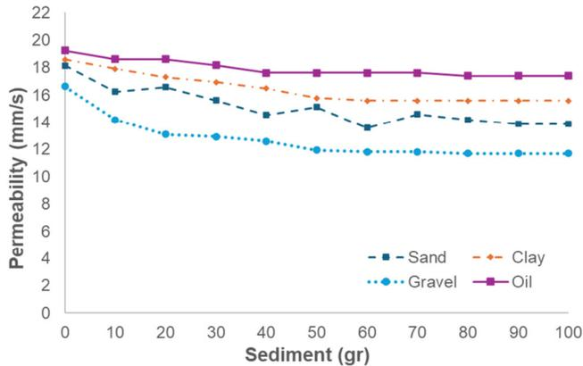
Fig. 3. Permeability test of PC with aggregate size 12.5–19.1 mm using different sediments.
