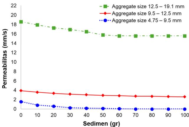
Fig. 2. Permeability test using clay sediment.
