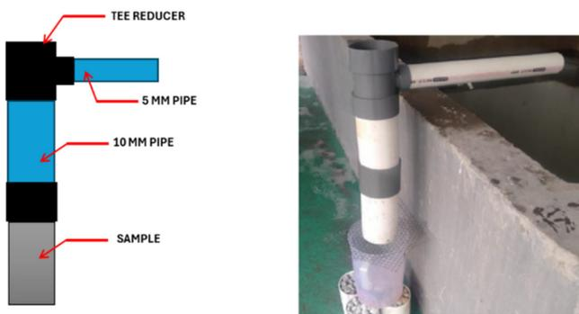
Fig. 1. Test apparatus setup.
