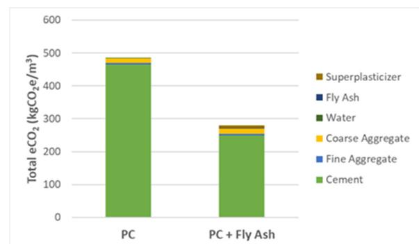
Fig. 4. Comparison of eCO<sub>2</sub> of concrete with and without Fly Ash.
