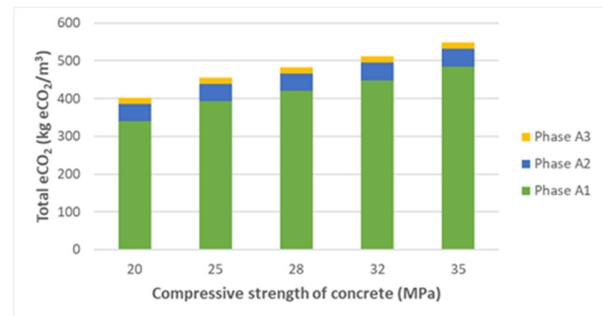
Fig. 2. Total eCO<sub>2</sub> for each concrete grade.
