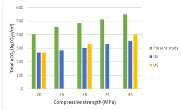
Fig. 3. Comparison of eCO<sub>2</sub> in concrete: Present Study vs. UK vs. US.
