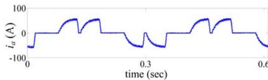
Fig. 18. Stator phase current when the machine is supplied LCI and dc-link pulsing method is applied ( $f = 3$  Hz,  $I_{dref} = 48$ ).
