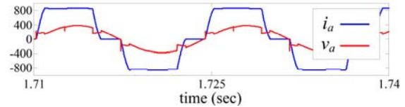
Fig. 14. Stator phase ‘a’ current and voltage waveforms when the machine is supplied from the conventional three-level LCI ( $\omega=2100$  rpm,  $I_{dc}=850$  A).
