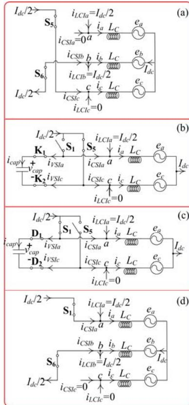
Fig. 6. CSI and VSI equivalent circuits for: (a) normal conduction before commutation between phases 'a' and 'c' starts, (b) mode 1, (c) mode 2 and (d) mode 3.
