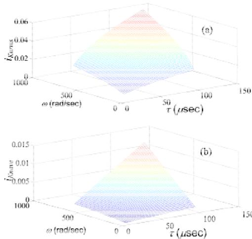
Fig. 9. Current ratings of VSI switches as a function of  $\tau$  for different motor speeds ( $C_{dc}= 500 \mu\text{F}$ ), (a)  $i_{KNrms}$  and (b)  $i_{KNave}$ .
