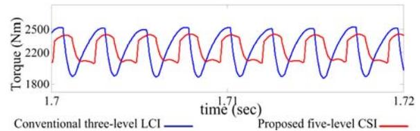
Fig. 16. Electromagnetic torque of WFSM ( $\omega=2100$  rpm).
