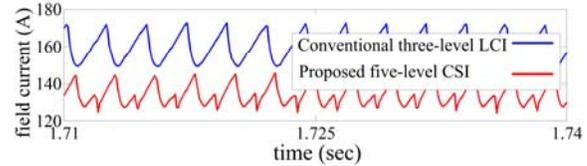
Fig. 15. Field current of WFSM ( $\omega=2100$  rpm).
