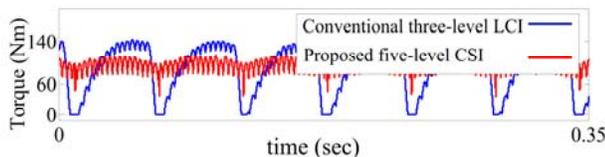
Fig. 19. Machine electromagnetic torque ( $f = 3$  Hz).
