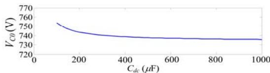
Fig. 11.  $V_{C0}$  as a function of  $C_{dc}$  ( $\tau=70 \mu\text{sec}$ ) for rated operating condition.
