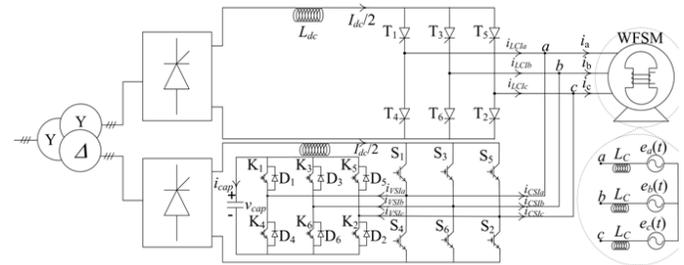
Fig. 1. Proposed five-level CSI for WFSM drives.
