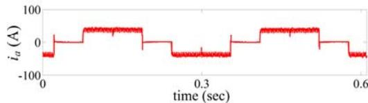
Fig. 17. Stator phase current when the machine is supplied by CSI and LCI is turned off during start-up or low-speed operating conditions ( $f = 3$  Hz,  $I_{dref} = 38$  A,  $C_{dc} = 500$   $\mu$ F,  $\tau = 70$   $\mu$ sec).
