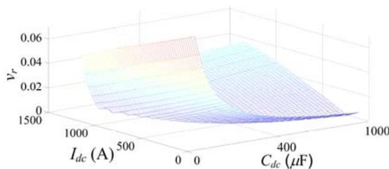
Fig. 10. DC capacitor voltage ripples as a function of  $C_{dc}$  ( $\tau=70 \mu\text{sec}$ ).
