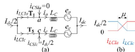
Fig. 4. The loop created by the simultaneous conduction of  $T_1$  and  $T_5$  (commutation interval '1' in Figure 3) and (b) current variations.
