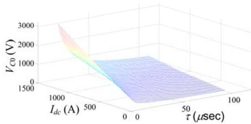
Fig. 8.  $V_{C0}$  as a function of  $\tau$  under different operating conditions ( $C_{dc}=500 \mu\text{F}$ ).
