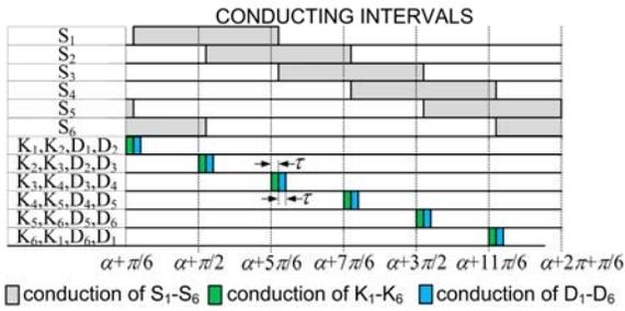
Fig. 5. Switching pattern of CSI and VSI devices.  $\alpha + \pi/6$  corresponds to point B in Figure 2a.
