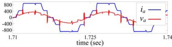
Fig. 12. Stator phase ‘a’ current and voltage waveforms when the machine is supplied from the five-level current-source inverter ( $\omega=2100$  rpm,  $I_{dc}/2=445$  A,  $C_{dc}=500 \mu\text{F}$  and  $\tau=70 \mu\text{sec}$ ).
