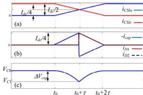
Fig. 7. Waveforms related to commutation between phases 'a' and 'c', (a)  $i_{csta}$  and  $i_{cstc}$ , (b)  $i_{D1}$  and  $i_{D2}$ , (c)  $v_{cap}$ .
