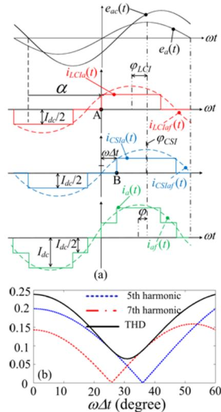
Fig. 2. (a)  $i_{LCIa}(t)$ ,  $i_{CSIa}(t)$  and  $i_a(t)$  waveforms and their corresponding fundamentals and WFSM phase and line voltages, (b) 5<sup>th</sup> and 7<sup>th</sup> harmonic amplitudes (relative to fundamental) and THD for the phase current  $i_a$  as a function of  $\omega\Delta t$ .
