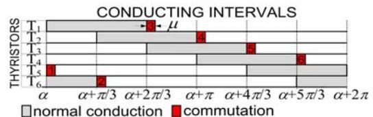
Fig. 3. Switching pattern of LCI.  $\alpha$  corresponds to point A in Figure 2a
