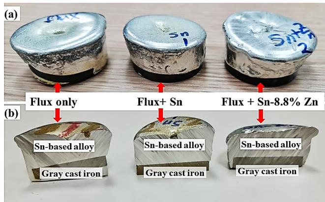
Fig. 2. (a) Sn-based alloy/GG25 gray iron bimetal composite specimens, (b) cross sections of three specimens.
