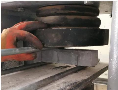
Fig. 8. Testing a cubic concrete sample.
