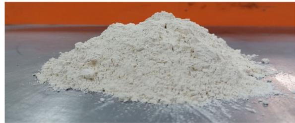
Fig. 2. Glass powder used in this work.
