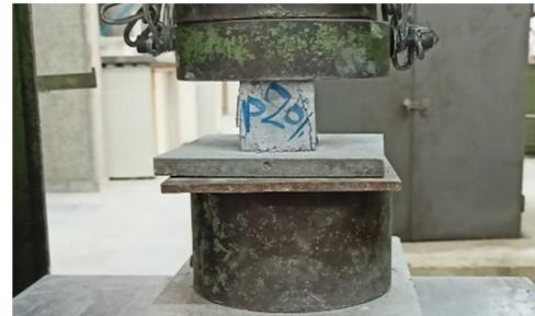
Fig. 5. Testing a prismatic concrete sample.
