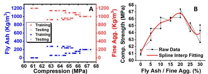
Fig. 2. Relationships between the FA and S content as mixed proportions against the compressive strength of AACMs: (A) Comparison between the selected trained/tested datasets used in the supervised ML, (B) experimental data of FA/S ratio against compression fitted by spline interpolation using ORIGIN.
