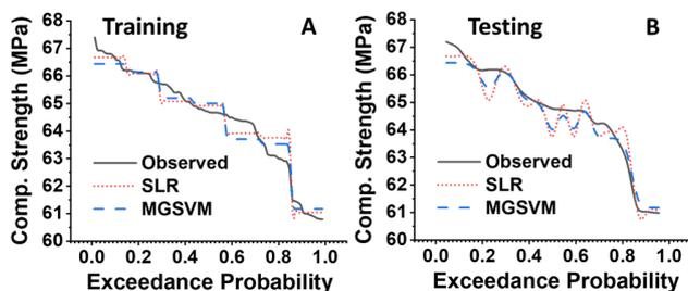
Fig. 4. Observed vs. predicted compressive strength showing the exceedance probability of the ML models.
