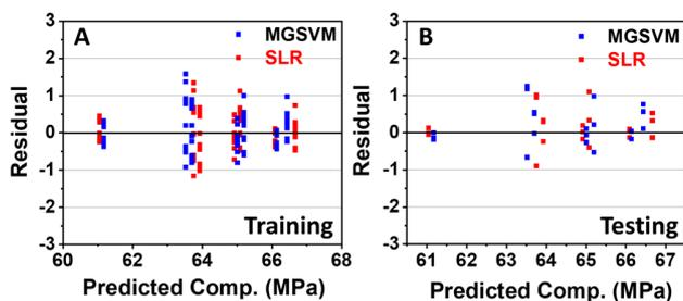
Fig. 6. Residual statistical analysis showing SRL and MGSVM accuracy: (A) Training datasets showing the low residual range of  $\pm 1$  indicating high accuracy of the models, (B) testing datasets confirming the models' ability to estimate experimental results with similar trained model high accuracy of  $\pm 1$ .
