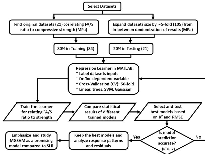
Fig. 1. Flowchart for developing and selecting the optimal ML models for accurate prediction of compressive strength correlated with FA/S ratio.
