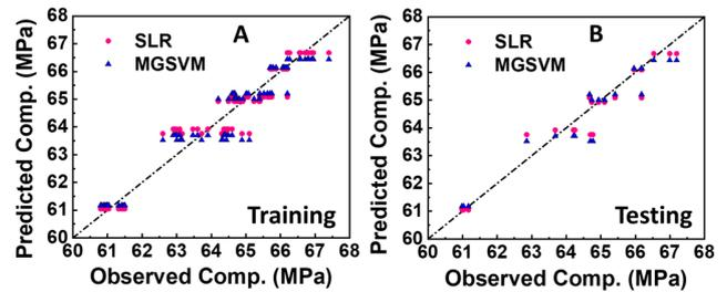
Fig. 5. Observed vs. predicted compressive strength of AACM composites showing the prediction accuracy of the built ML models: (A) training, (B) testing.
