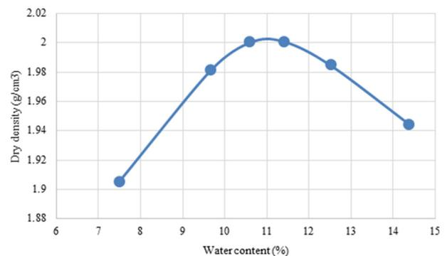
Fig. 3. Curves of water content and maximum dry density.
