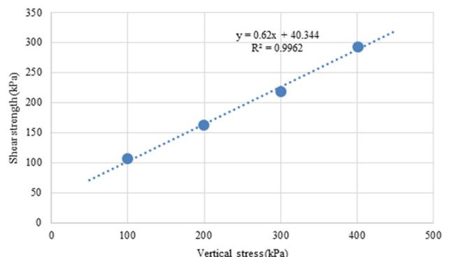
Fig. 4. Relationship between shear strength and vertical pressure.
