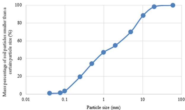
Fig. 2. Gradation curve of bottom slag particles.
