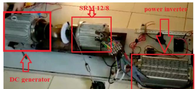
Fig. 8. Dynamic torque test bench.
