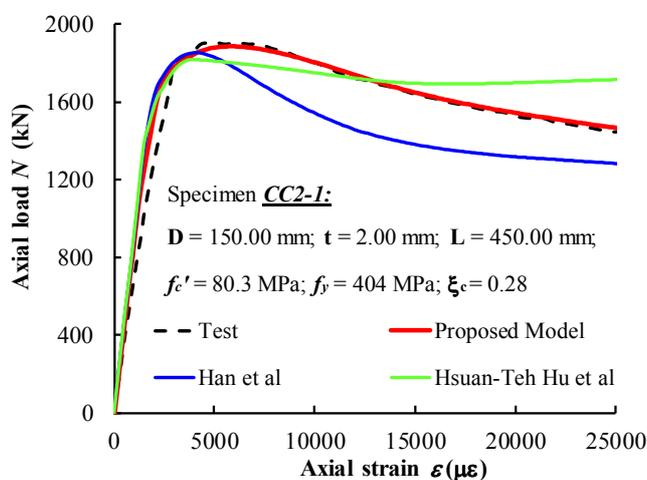
Fig. 8.  $N - \varepsilon$  curves of the CFST column with thin-walled and high-strength steel.
