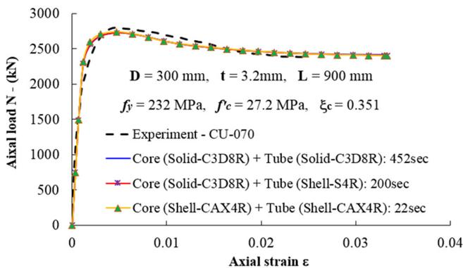
Fig. 5. Influence of the meshing and element types.
