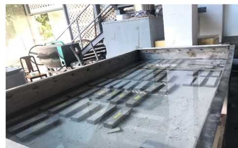
Fig. 5. The samples were cured for 27 days in water.
