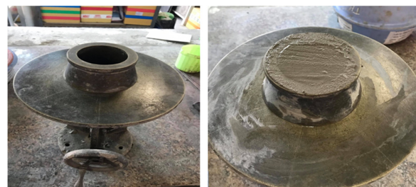
Fig. 1. The fresh mortar into the cone shape of the flow table.
