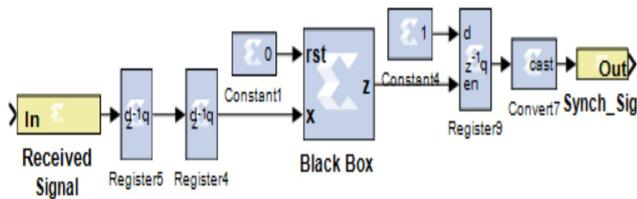
Fig. 12. Sync detector, as views using the Xilinx System Generator.
