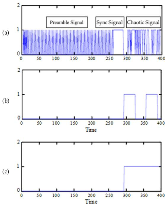
Fig. 13. Simulated test of the sync stream module: (a) Preamble data, sync data, and chaotic signal, (b) synch signal is detected, (c) synch signal is constant.
