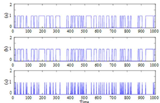
Fig. 4. Simulated results: (a) Binary random generator (Bernoulli), (b) delayed data by one sample, (c) rising and falling edge detections.
