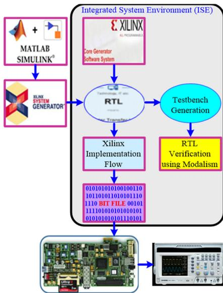
Fig. 14. Block diagram of the design procedure.
