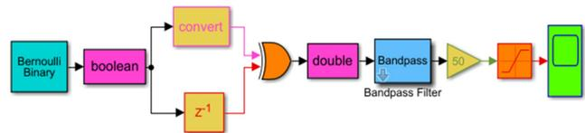
Fig. 3. Clock recovery Simulink model.
