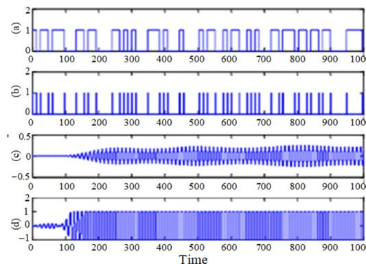
Fig. 6. Simulated test of clock recovery: (a) Binary random generator (Bernoulli), (b) rising and falling edges, (c) bandpass filter response, (d) recovered clock.
