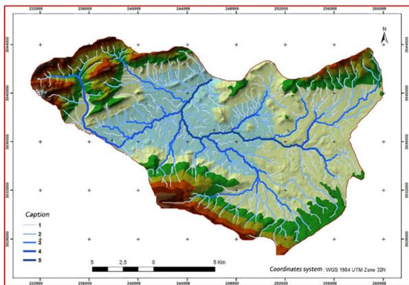
Fig. 12. Hydrographic network of the watershed of Batna with flow order (source: authors using DTM on images from the National Institute of Cartography and Teledetection)
