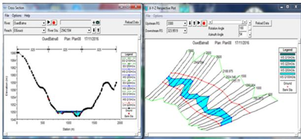
Fig. 20. Oued Batna valley geometry using HEC RAS software
