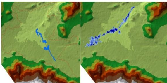
Fig. 21. Spots representing flood areas on Oued Batna and Oued El Gourzi valleys based on a 100-year frequency flow - HEC GeoRAS (postRas)
