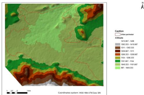
Fig. 17. Creation of DTM of Batna city watershed
