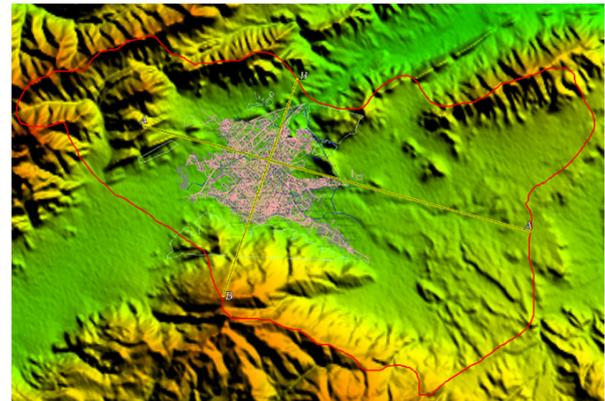
Fig. 5. Topography of the watershed of Batna city (source: authors using DTM on images from the National Institute of Cartography and Teledetection)
