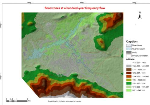
Fig. 22. Map of the flood hazard of the city of Batna obtained using- Hec RAS – DTM
