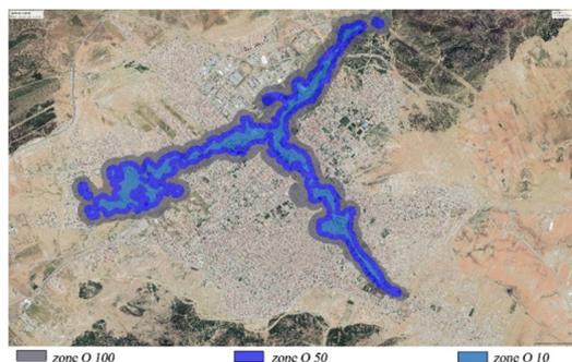
Fig. 25. Satellite image of flood areas related to the valleys Oued Batna and Oued El Gourzi using Google Earth Pro (Screenshot from Google Earth, Image © 2019 Maxar Technologies CNES/Airbus)
