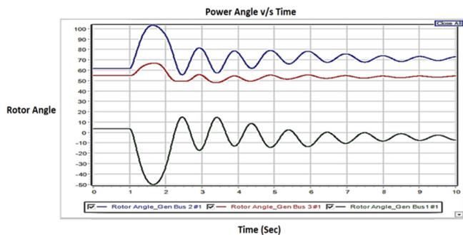
Fig. 1. Rotor angles of three generators for a three phase short circuit balanced fault on the transmission line between bus 5 and bus 7 at 1.0s.
