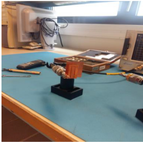
Fig. 6. The antenna in S-parameter testing
