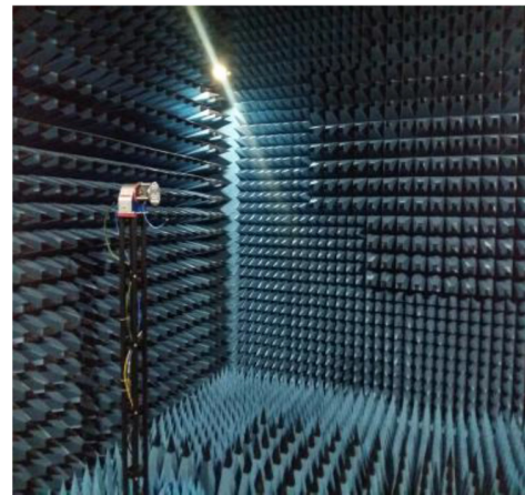
Fig. 8. The proposed antenna prototype during testing in the anechoic chamber
