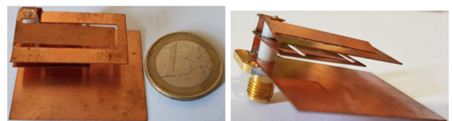
Fig. 5. The prototype of the multi-band antenna
