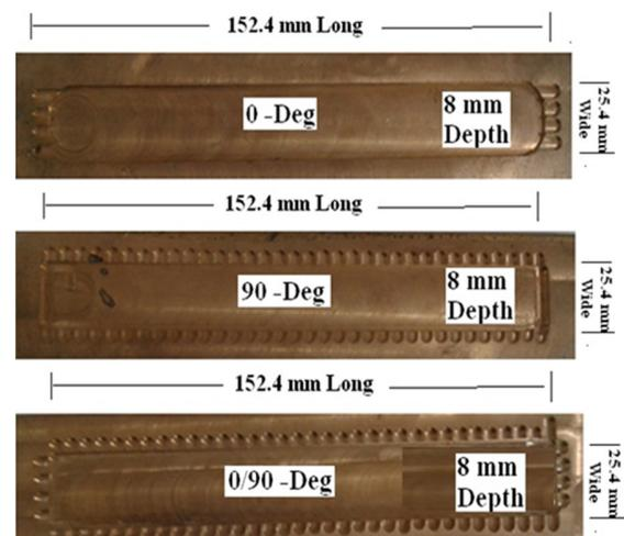
Fig. 2. Mold's design
