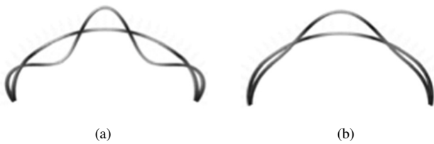
Fig. 8. An example of elastic buckling mode shapes for Profile E: (a) deep burial and (b) zero soil cover.
