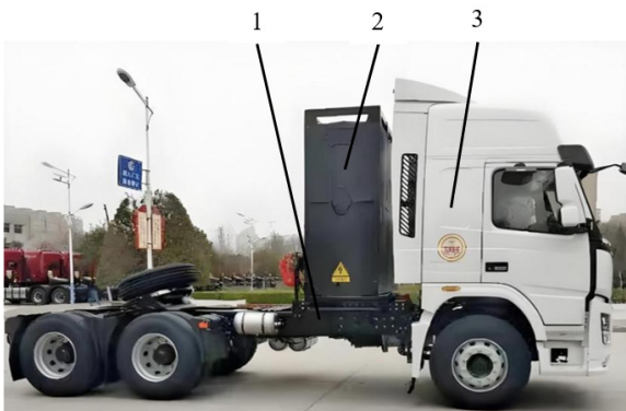
Fig. 1. A pure electric heavy-duty truck with a rear-mounted battery system, showing: (a) chassis frame, (b) power battery assembly, and (c) cab.
