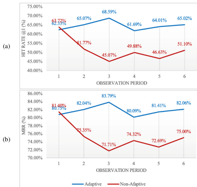
Fig. 7. Channel recommendation performance over time for adaptive and non-adaptive configuration: (a) Hit Rate @1, (b) MRR.
