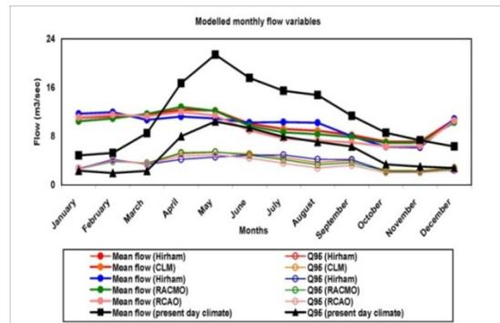
Fig. 8. The projected mean monthly environmental flow (Q95) and total stream flow regime under A2-emission scenario
