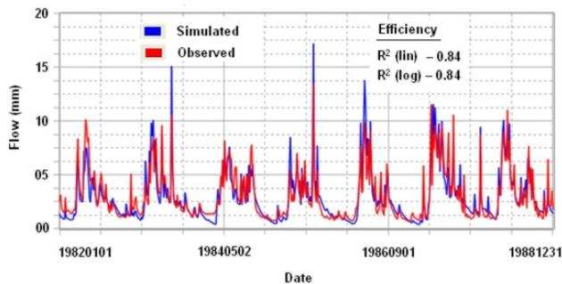
Fig. 2. Graphical comparison of observed and simulated daily hydrograph at the gauge station (St Johann i.T) of the Kitzbüheler Ache catchment for calibration period (1983-88).
