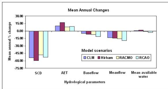
Fig. 10. The relative mean annual changes in snow cover duration (SCD), actual evapotranspiration (AET), baseflow (BF), total flow and total available water under A2-emission scenario.
