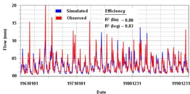
Fig. 3. Graphical comparison of observed and simulated daily hydrograph at the gauge station (St Johann i.T) of the Kitzbüheler Ache catchment for validation period (1961-90).
