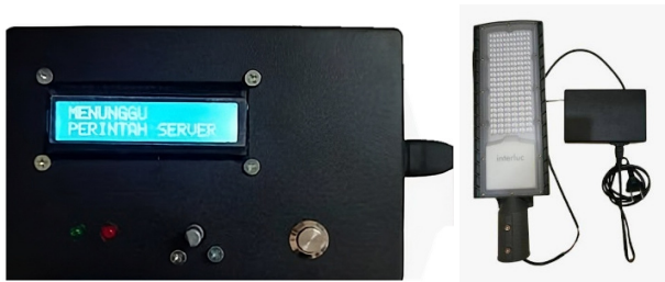
Fig. 2. Prototype street light using XBee.
