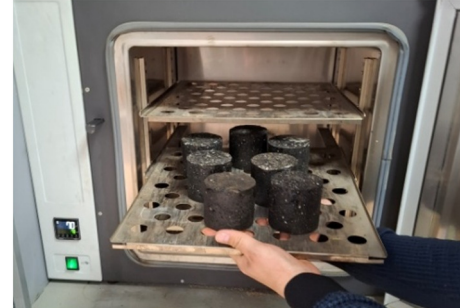
Fig. 1. Testing of asphalt concrete samples.
