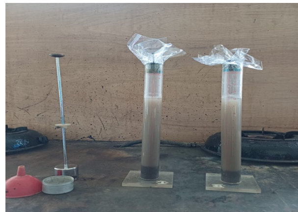
Fig. 3. Sand equivalent test.
