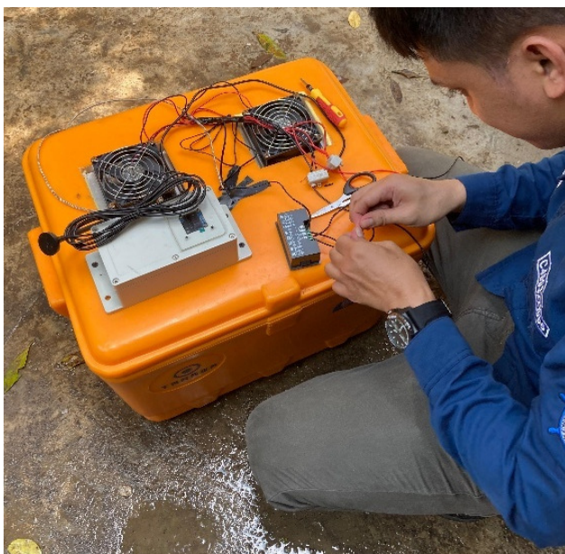
Fig. 4. Experimental prototype configuration of the hybrid ice-Peltier smart fish hold and IoT monitoring system.
