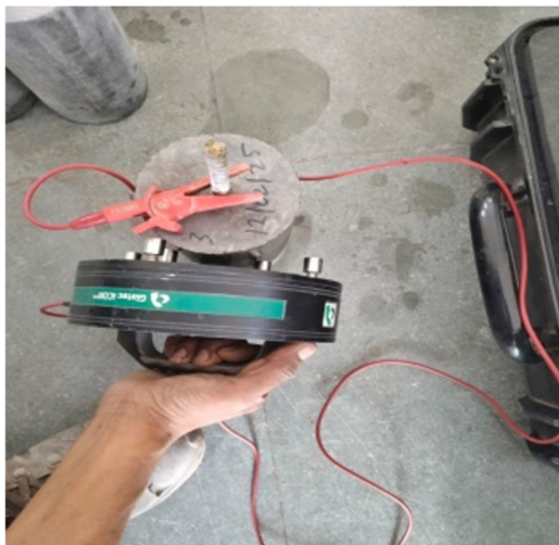
Fig. 3. Half-cell potential measurement on concrete specimen.
