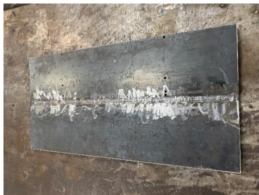
Fig. 3. GTAW-SMAW hybrid welding process on the capping pass.
