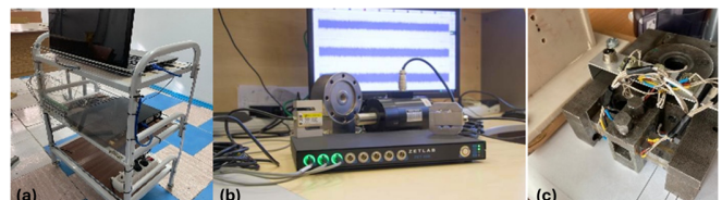
Fig. 16. Experimental setup for determining cutting forces.
