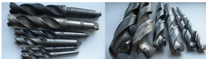
Fig. 14. Prototypes of double-edge twist drills without a transverse edge.
