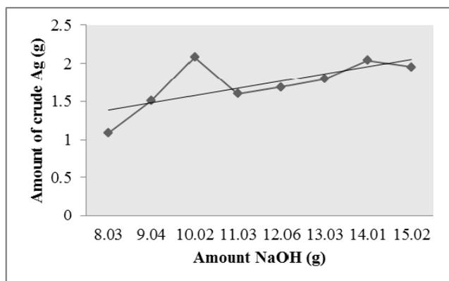
Fig. 8. Relationship between amount of alkaline reagent used and the amount of crude silver recovered
