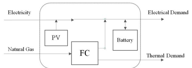
Fig. 1. Residential building multi-carrier energy system
