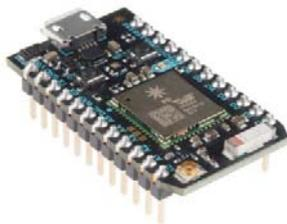
Fig. 3. Particle photon kit
