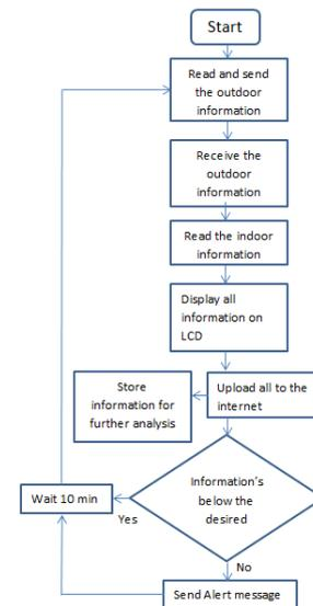
Fig. 8. System operational flow chart
