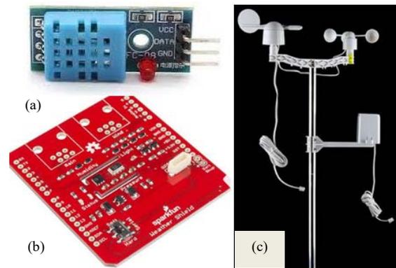
Fig. 4. Weather shield, DHT11, and wind-rain sensor.
