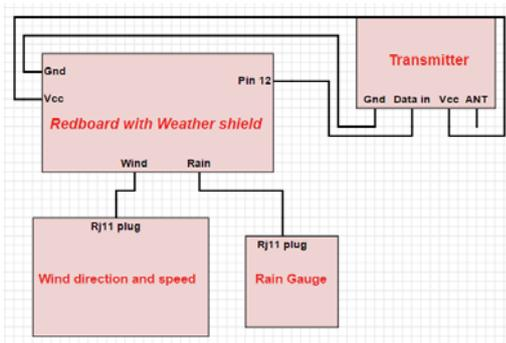
Fig. 6. Outdoor practical connection between the different circuitry
