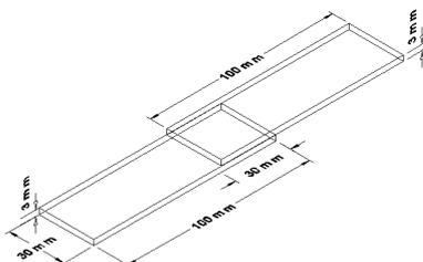
Fig. 1. Sample geometry for the welding process
