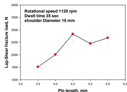
Fig. 3. Variation of lap-shear fracture load with pin length
