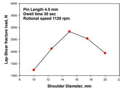
Fig. 5. Variation of lap-shear fracture load with shoulder diameter
