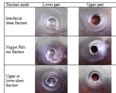
Fig. 6. Photographs of failure surfaces show the typical failure modes of test specimens.
