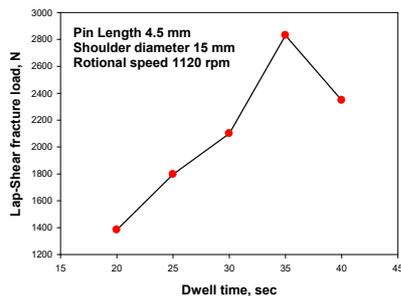
Fig. 4. Variation of lap-shear fracture load with dwell time
