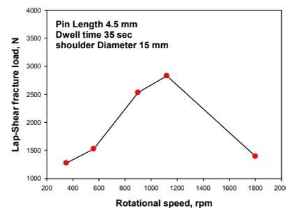
Fig. 2. Variation of lap-shear fracture load with rotational speed
