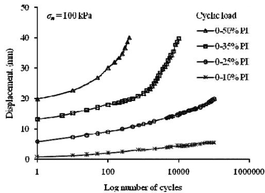
Fig. 4. Displacement-log number of load cycles relationships.
