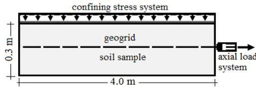
Fig. 1. Pull-out test device.
