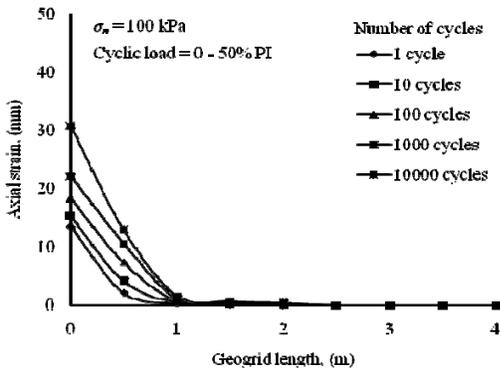
Fig. 6. Change in axial strain with number of load cycles.
