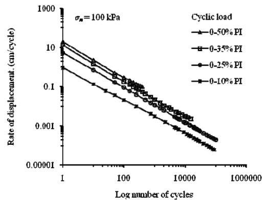
Fig. 5. Rate of displacement-log number of load cycles relationships.
