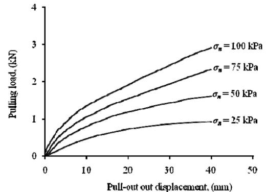
Fig. 2. Load-displacement relationships of the geogrid.
