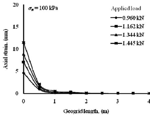
Fig. 3. Axial deformation along the geogrid.
